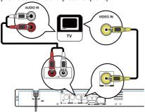
1. Connect a composite cable from the VIDEO OUTPUT jack and analog AUDIO OUTPUT jacks on this product to the video input jack (yellow) and audio input jacks (white/red) on the TV.
